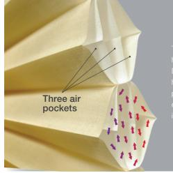
The patented honeycomb design of Duette Architella Shades has three distinct air pockets for superior energy efficiency and increased insulation.
