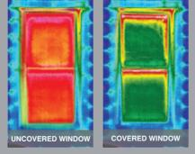
The infra-red images show a covered window on the right demonstrating ignificantly improved energy savings ersus the uncovered window on the left
